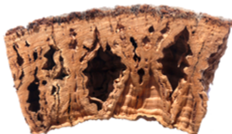
Figure 16 – Lièges excessivement poreux
